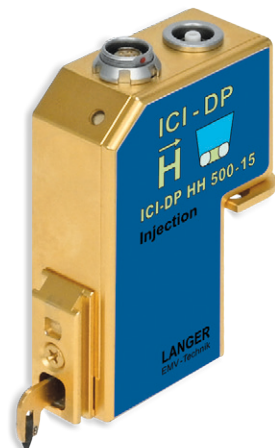
ICI-DP HH500-15 Double Pulse Magnetic Field Source
